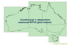
For points outside of the *NTv2 national conformal + distortion transformation grid* above, such as Cocos / Keeling and Christmas Islands, **7-parameter similarity (Helmert) transformation (conformal) [EPSG: 8048]** has been employed.
