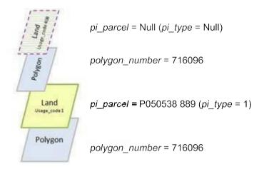
Easements are a Cadastral Family and comprise a separate polygon where the easement does not encumber the entire lot/land parcel SCDB data. In this example, two (2) features will be provided, one for each usage type. Note: SCDB rules allow easement polygons to overlap other cadastral polygons.
