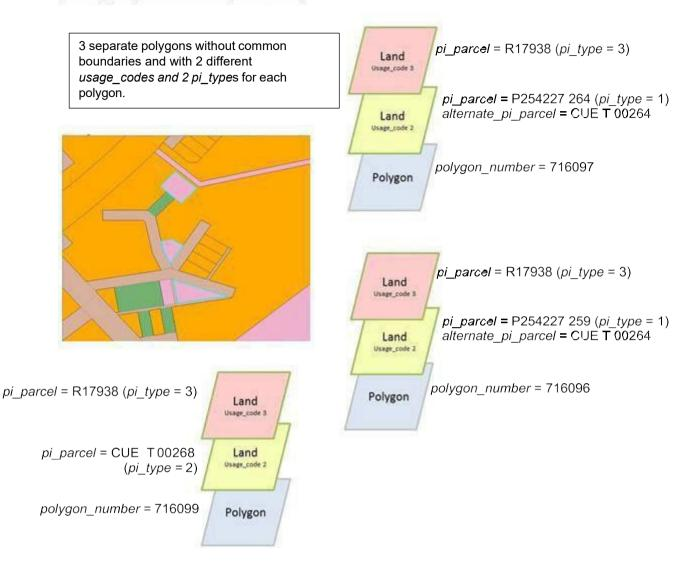
Six (6) separate features will be created for the three (3) highlighted geometries (– one for each Usage Code.
