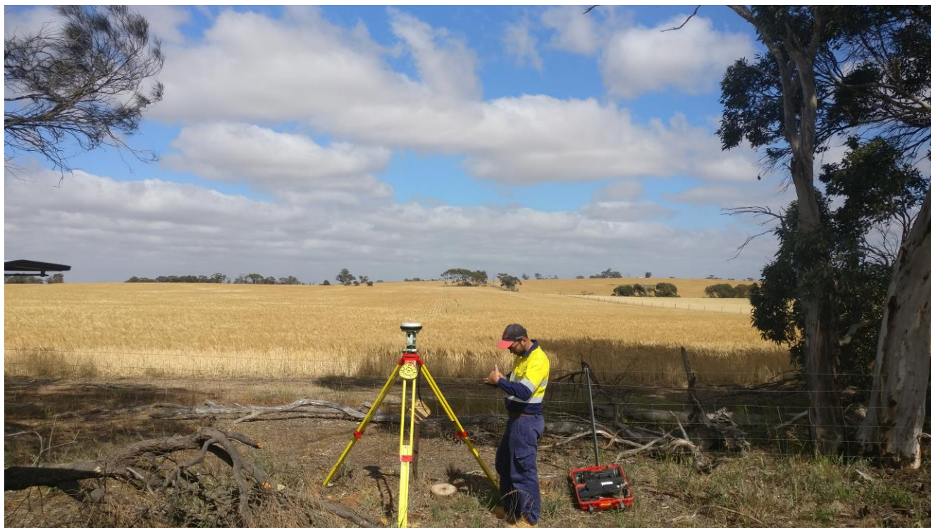
GNSS survey to improve regional geodetic network.
